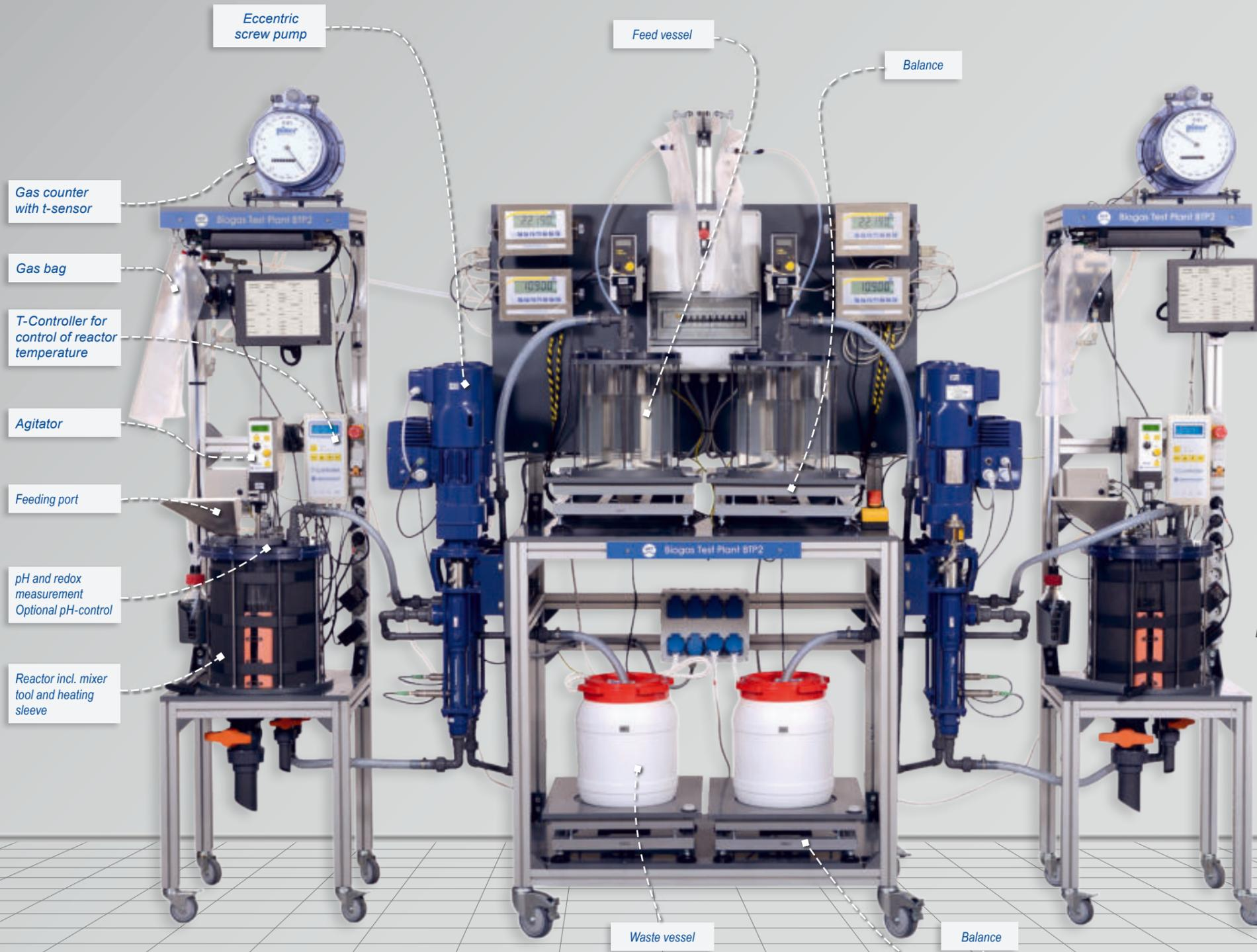
The individual BTP modules can also be equipped with eccentric screw pumps.
