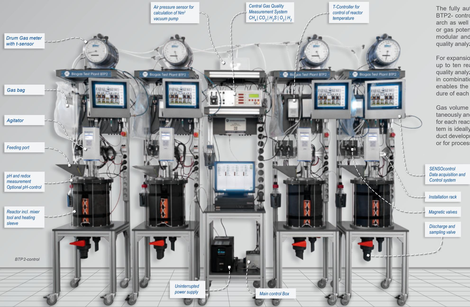
The fully automated bioreactor plant BTP2- control is mainly used in research as well as for practical substrate or gas potential tests. This system is modular and equipped with one gas quality analyzer module.
